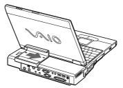
3 Slide the floppy disk drive in the direction of the arrow until it locks into place, then connect the floppy disk drive to the docking station with the floppy disk drive cable.
